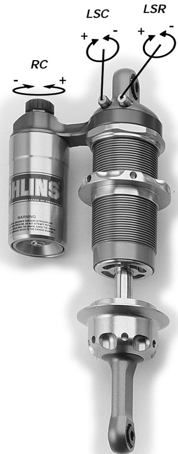
Figure 6. Standard external adjusters. - = soft. + = hard.
