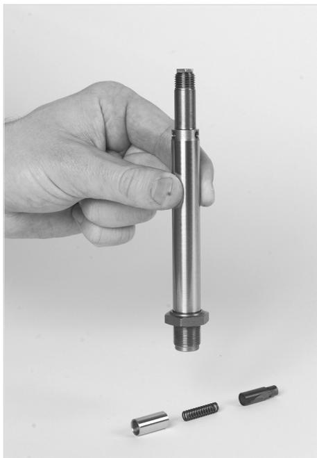
✓ Remove the end eye from the shaft.
