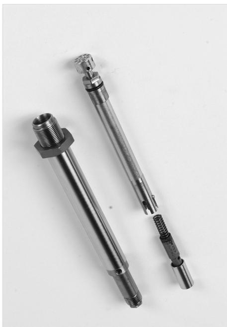
✓ Remove the entire adjuster assembly mechanism.
